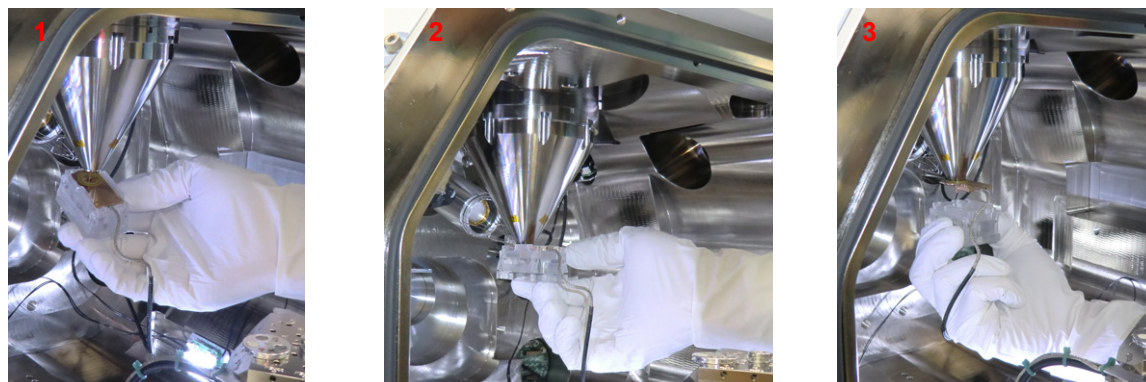
FIGURE 7-4: Directional GAD detector installation
