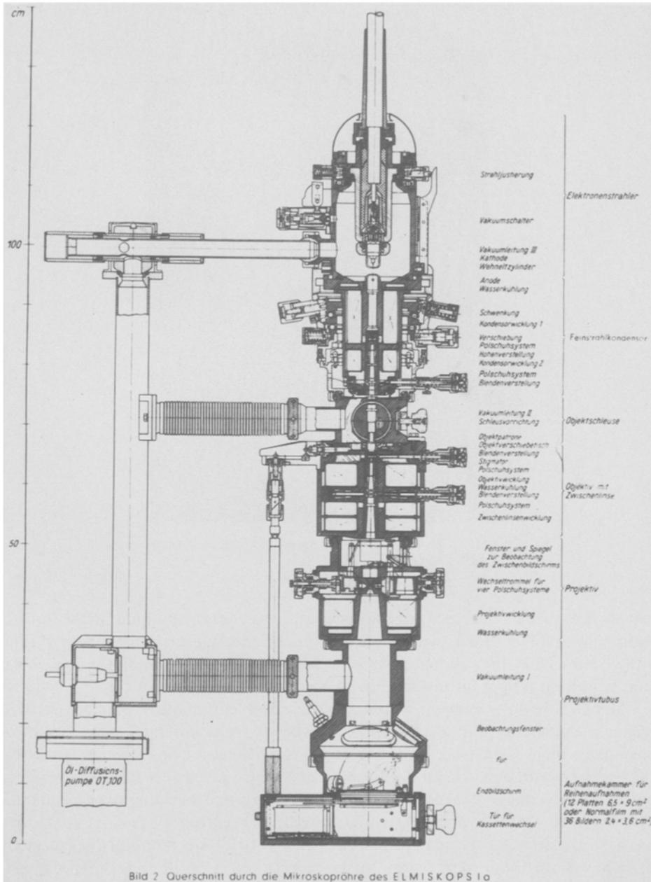
**Fig. 12.** The first serially produced 100 kV-Electron microscope with two condenser lenses for "small region radiation" (Siemens) (left) cross-section; (right) general view (23).
