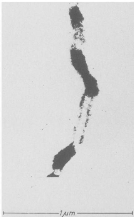
**Fig. 9.** Iron Whisker ( $U = 79$  kV,  $M_{el} = 3100\times$ )
