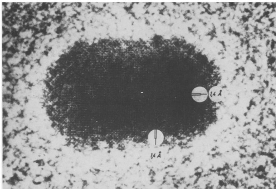
**Fig. 15.** Plate-like gold crystal lattice planes with a separation of 0.14 nm, taken with axial illumination. ( $U = 100$  kV,  $M_{el} = 800,000\times$ ); taken (1976) by K. Weiss and F. Zemlin with the 100 kV transmission electron microscope with single-field condenser objective at the Fritz-Haber-Institut of the Max-Planck-Gesellschaft.
