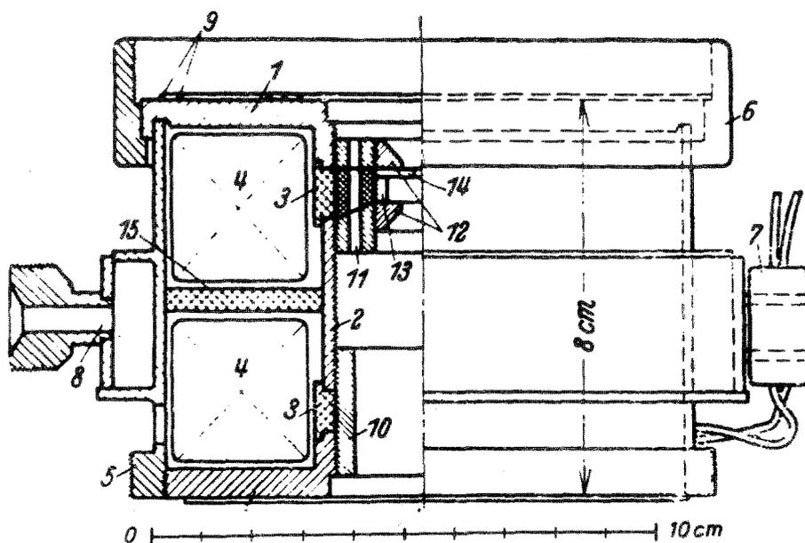
Fig. 4. Cross-section of the first polepiece lens (14,15).
