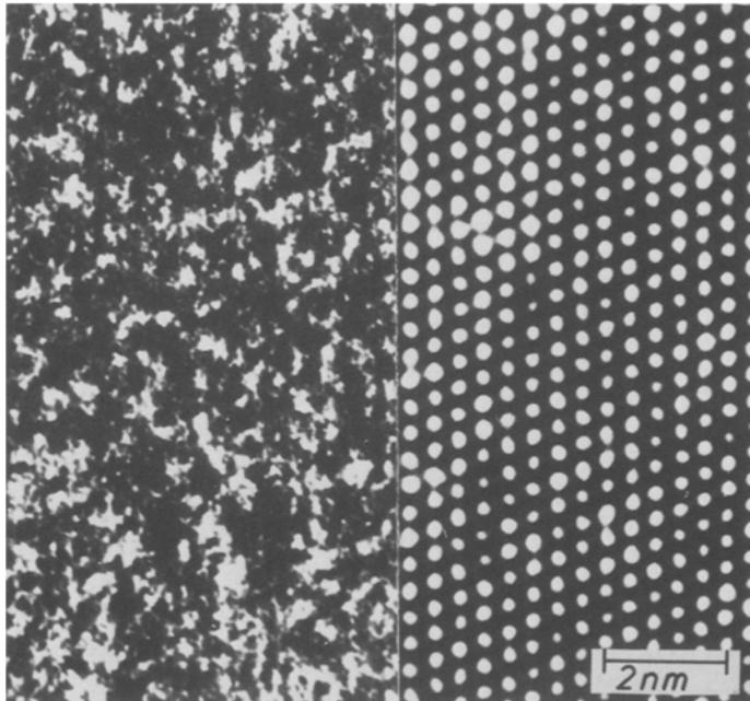
**Fig. 17.** Paraffin crystal (left: image taken with minimum dose, right: superposition of 400 sub-regions of the left image by means of the computer. (25).
