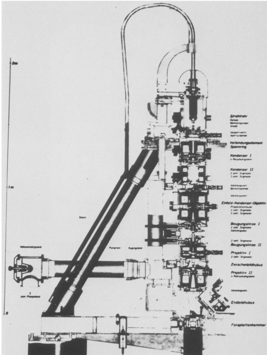
Fig. 13. 100 kV-Electron microscope with single-field condenser objective (cross-section) (24).
