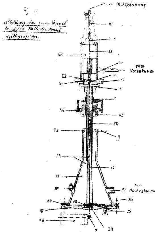
Fig. 1. Sketch by the author (1929) of the cathode ray tube for testing the imaging properties of the non-uniform magnetic field of a short coil (4,5).
