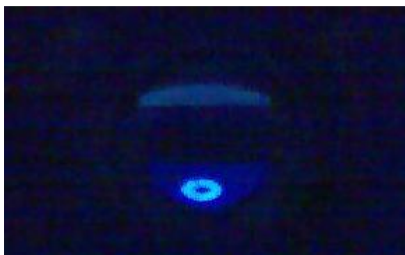
Figure 3: FEG Emission Pattern
