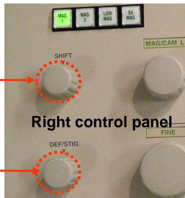
4. Go magnification at least higher than 250k. Higher than 1M is recommended. Press “Cond stig” on the left control panel, in order to correct condenser astigmatism. Make the Ronchigram as round as possible with Def/Stig x/y. See below.
